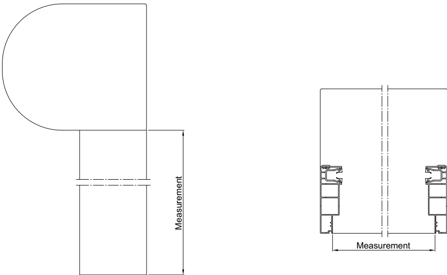
fig. 158: Measuring for retrofitting insect screens
