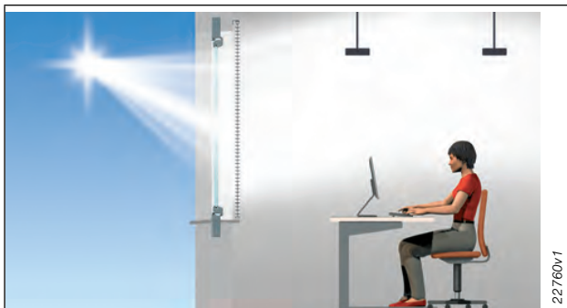
fig. 4: Principle of light guidance using daylight guiding venetian blinds
